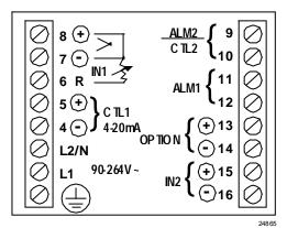
Figure 6—External Wiring Diagram
